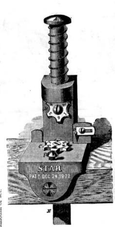
The points are all of different sizes, and are numbered from 1 to Prominent among its advantages is the fact that it can be operated wholly by the foot by means of a treadle, thus leaving the hands The striking part and the anvil, or portion which receives the blow, are star-shaped and to guide and manipulate the Saw and are designed to set diff similar in construction.
